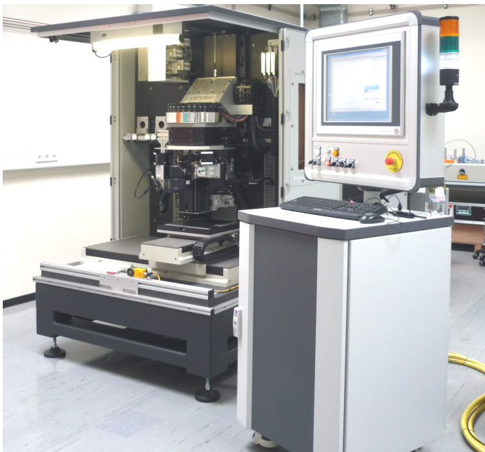
SP450-TO, showing large turret optics & unparalleled workstation access with large safety doors double folding entirely to the rear.
