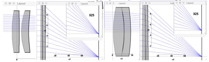
If we allow 3 elements, the world is pretty much our oyster. Such a Cooke triplet can correct all five  $3^{rd}$  order Siedel aberrations, as well as colour if more than one material is used, for e.g. for UV wavelengths UVFS & CaF2.
