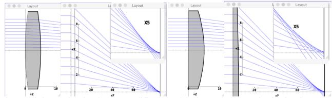
...or better, with the same lens the other way round! First lesson then; the most highly curved surface has always to be towards the most distant conjugate, in this case infinity. Slightly better again is a 'best form' lens with about 85% of the power in the surface facing the collimated beam, but the gain is small over the correctly orientated plano-convex:-
