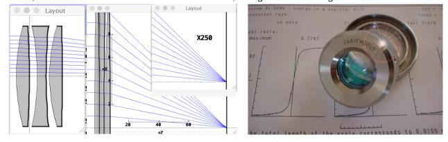
Once aberrations are reduced beyond a certain point, they are no longer relevant & the lens becomes 'diffraction limited', with performance determined by the wave nature of light; see Optec Technote RA/E/05. Giant tomes have been written on lens design, nowadays made relatively easy by computers. However the most important step in any lens design remains to cleary define the objectives, which then might suggest one 'family' of lens types over another.
