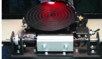
Thus, chucks need to be designed for the parts in question; in a general purpose machine interchangeable chucks can be useful. Left shows a combination part holder on Optec MicroMaster, with simple segmented flat circular chuck & vacuum 'V' groove for long thin cylindrical parts, typically catheters, on a simple motorized lathe; vacuum can be released for stepped rotation, or faced with slippery PTFE for continuous operations.
