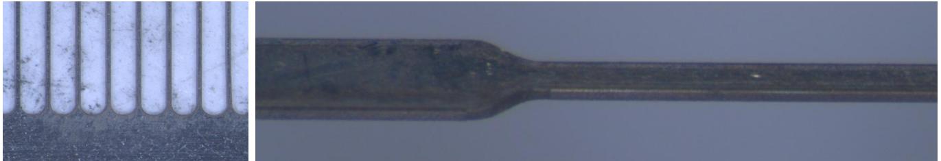
^ Cutting of 0.1 \text{ mm} thick Pt, feature pitch 650 \mu\text{m} ;
